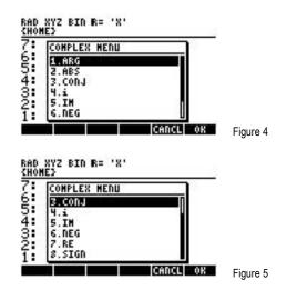
Two commonly used complex number functions are also on the 50g keyboard. ARG is the ORANGE shifted function of the  $\div$  key, and is accessed by pressing  $\frown$  \_ARG . ABS is the WHITE shifted function of the  $\div$  key and is access by pressing  $\frown$  \_ARG .
